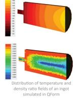
Simulation results from ProCAST program are imported into QForm V8 which allows forging simulations to be run based on the inherited characteristics of the casting simulation. It is possible to get joint virtual prototypes and sequences of casting and forging processes prior to product manufacturing. For simulation of heating and further forming of an ingot in QForm V8, finite element mesh is imported from ProCAST as well as temperature and porosity fields.
