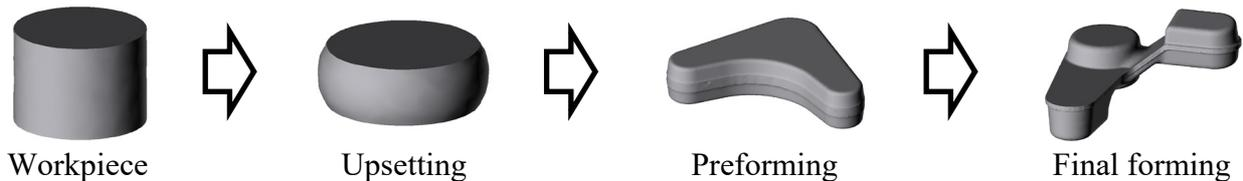
Figure 7. The sequence of forming process of the part «Lever»
