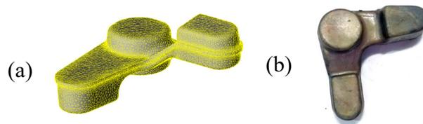
Figure 6. Finite element model (a) and the photo of forged part «Lever» (b)
