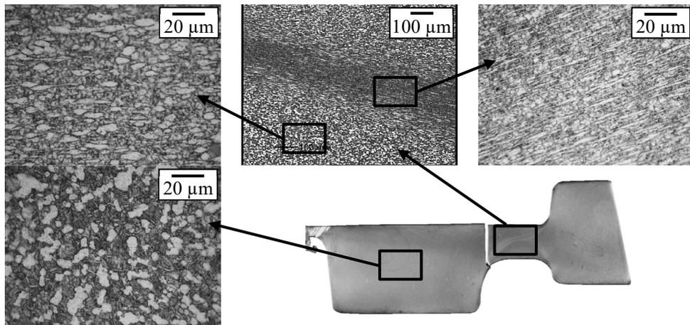
Figure 10. Macrograph and typical microstructure after final forming (Section 3)
