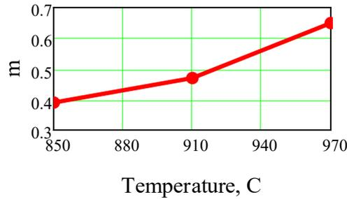
Figure 5. Temperature dependence of friction factor of TC11 alloy
