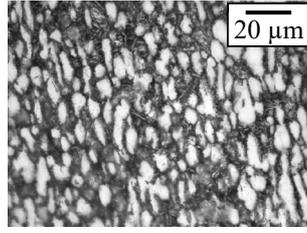
Figure 1. Initial microstructure of TC11 alloy
