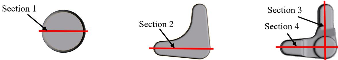
Figure 8. The scheme of crosscut sections in the part «Lever»
