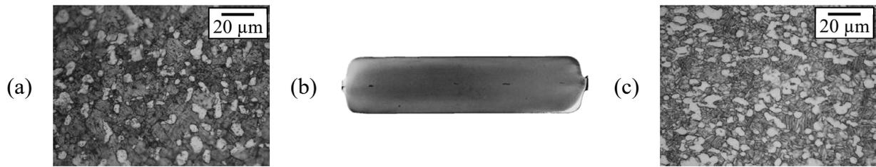
Figure 9. Typical microstructure (a) after upsetting (Section 1), macrograph (b) and typical microstructure (c) after preforming (Section 2)
