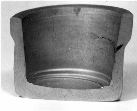
Figure 12. Photo of the cold forged cap with crack.
