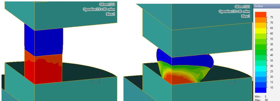
**Figure 2: Grain size distribution and deformation of bimetallic billet. (a) Initial shape, (b) shape after upsetting by 50%. Material is Ti6Al4V alloy, initial temperature is 850 C, initial grain size 5 mkm (top) and 80 mkm (bottom)**
