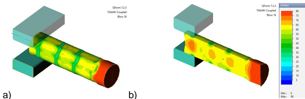
**Figure 1: Grain size distribution in a billet after cogging in 16 blows. (a) surface, (b) crosscut. Material is Ti6Al4V alloy, initial temperature is 850 C, initial grain size 80 mkm**
