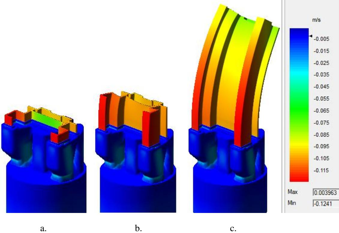
Fig. 6. Sequential steps of the material flow simulation in case of “rigid” dies. The beginning of the process (a), intermediate stage (b) and formation of the profile front tip (c).
