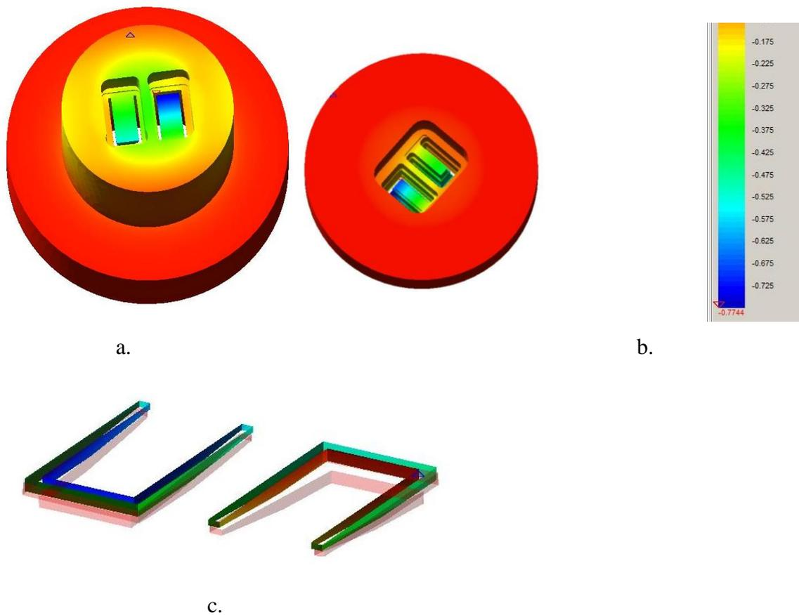
Fig. 2. The axial displacement of the die in mm shown from the container side (a) and from the outlet side (b) and local displacement of the bearing area (c). Colour scale shows the value of the displacement while pink contour in (c) is the deformed shape of the bearing magnified for better visibility.
