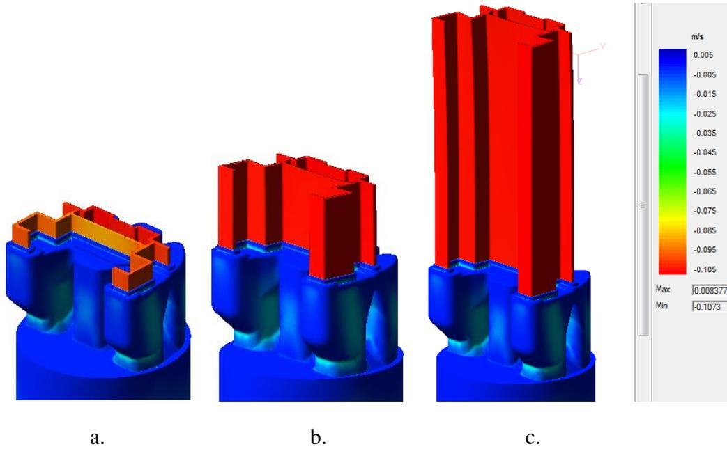
Fig. 9. Sequential steps of the material flow simulation in case of coupled simulation. The beginning of the process (a), intermediate stage (b) and formation of the profile front tip (c).
