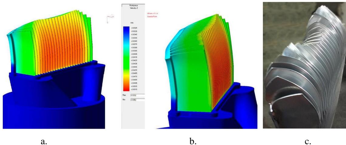
**Figure 5.** The shape of the front tip of the profile: (a) and (b) two different views obtained in simulation (axial velocity distribution) and (c) is the photo of a front tip in industrial extrusion
