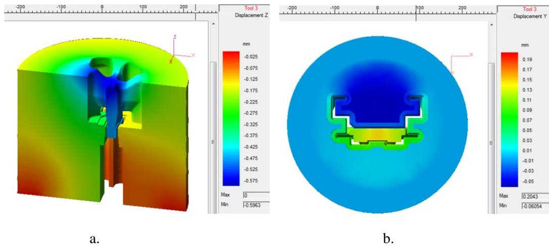
Fig. 7. Distribution of axial (a) and lateral (b) displacement in the crosscut of the tooling set
