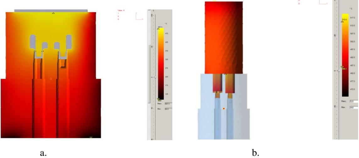
**Figure 10.** Temperature distribution in the die crosscut (a) and on the surface of the extruded material (b) after 50 seconds of the extrusion process obtained in coupled simulation.
