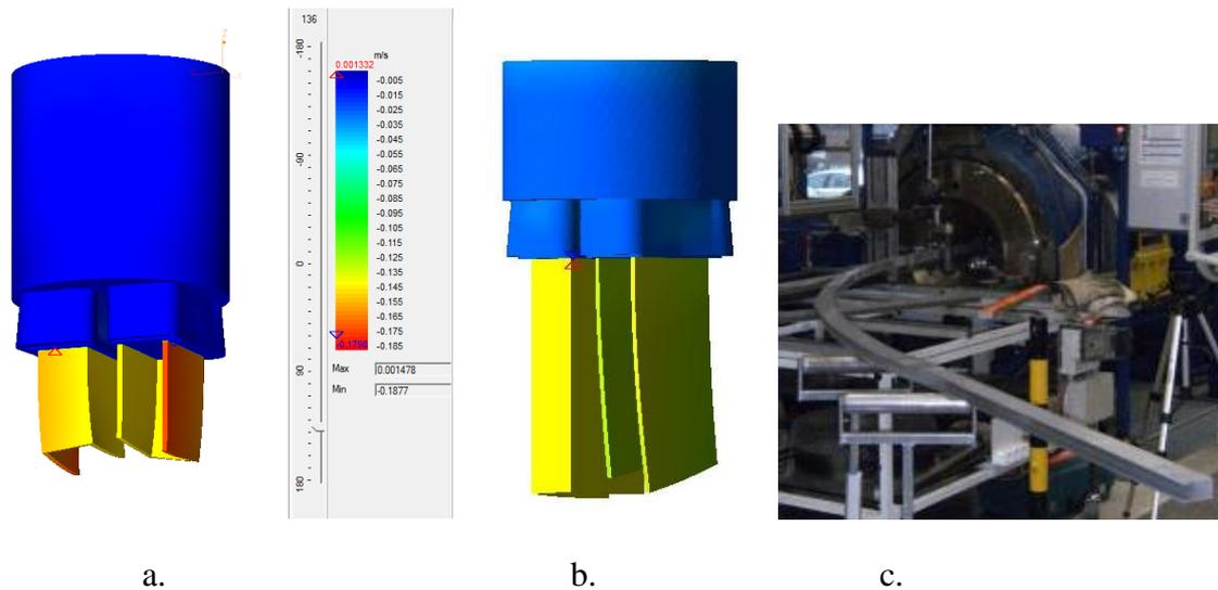
Fig. 3. Simulation of the test extrusion: with the rigid die both profiles go straight (a); with deformable die one profile bends in direction parallel to its legs (b); photo of the experiment [8] with one profile bending (c).
