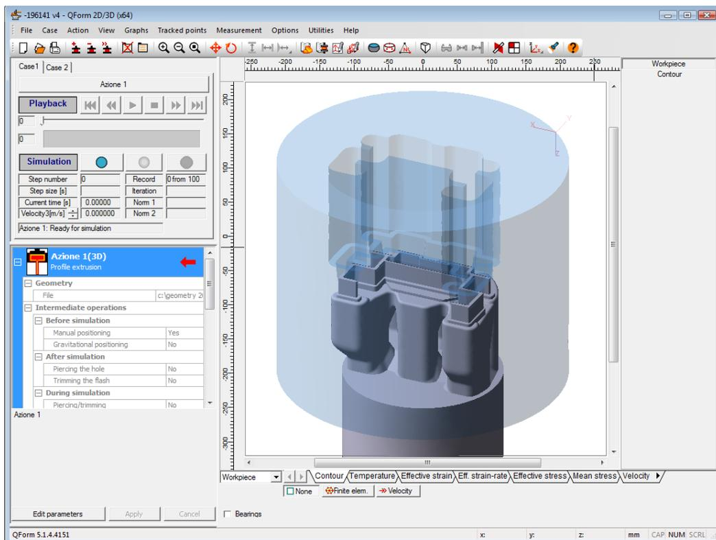
Fig. 5. The simulation setup in QForm-Extrusion with the die set while no container is shown. The material flow domain consists of 341405 nodes while tool set model consists of 241071 nodes
