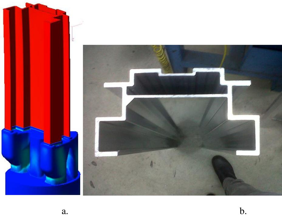
Fig. 10. Front tip of the profile in coupled simulation (a) and in reality (b).
