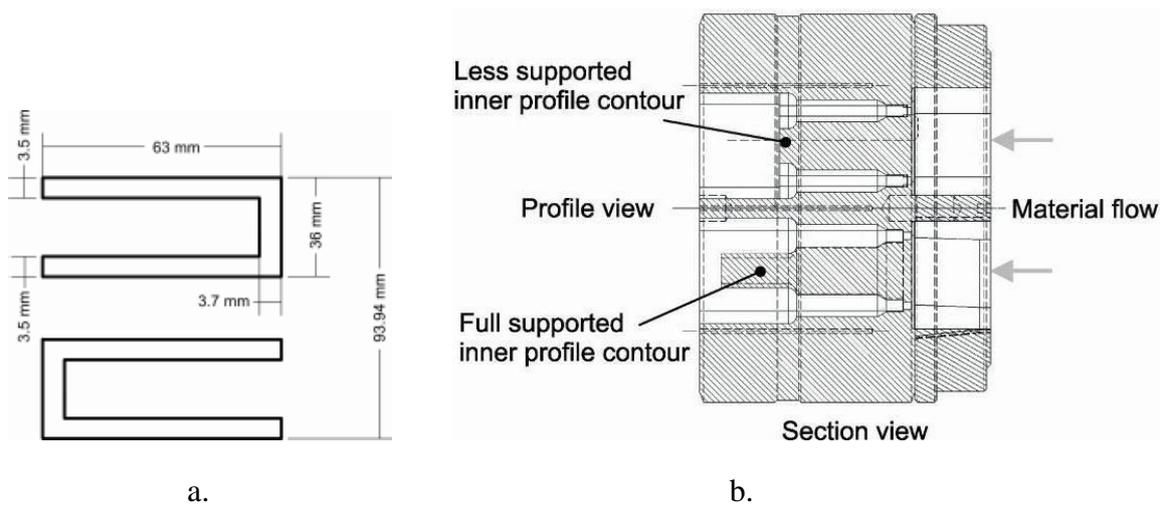
Fig 1. The scheme of the profiles used for the test (a) and crosscut of the die done through the tongues showing different support conditions (b). Both pictures are taken from [8].
