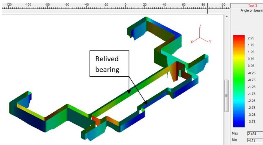
Fig. 8. Distribution of the inclination of initially straight bearing that was induced by elastic deformation of the die. The central part of the profile has got relieved bearing.
