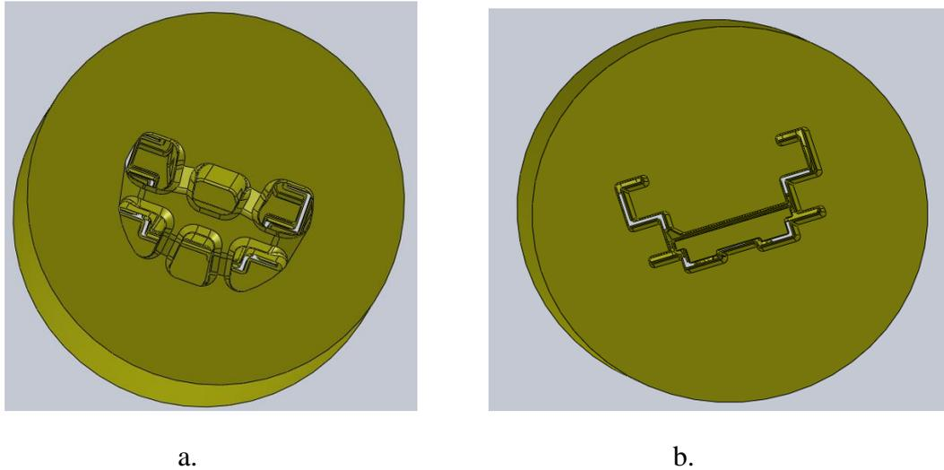
Fig. 4. The die for production of the profile shown from container (a) and exit (b) sides.
