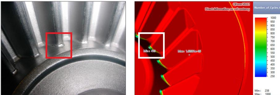
The crack in the die appeared in 400-500 cycles and its location predicted using proposed model with indication of the number of cycles till failure as 410
