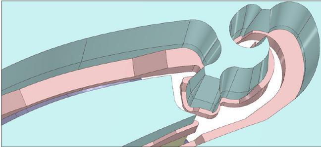
A solid bearings mode has also been added that allows the creation bearings with variable height values in solid models. The bearings are created automatically when they return to the parametrical model according to parameterization in the Bearing editor. Such a model takes the profile geometry characteristics into account and is more suitable for simulation of relief hogging as well as for further manufacturing of tooling set.
